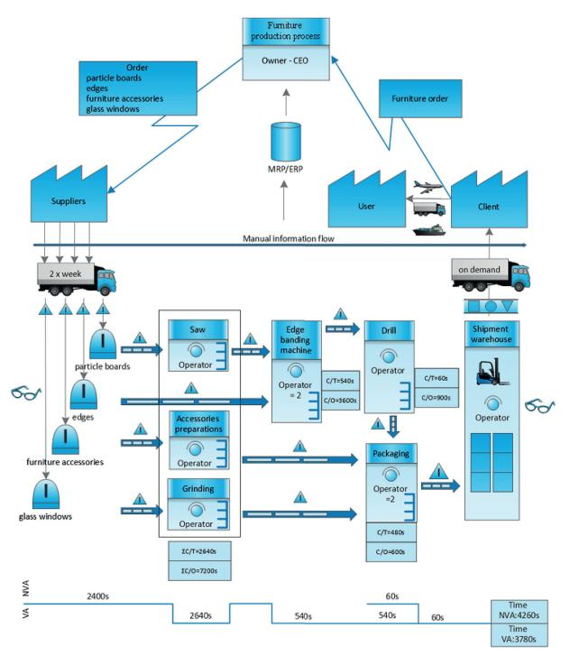
Figure 4. Value stream map of the furniture production process – initial state
