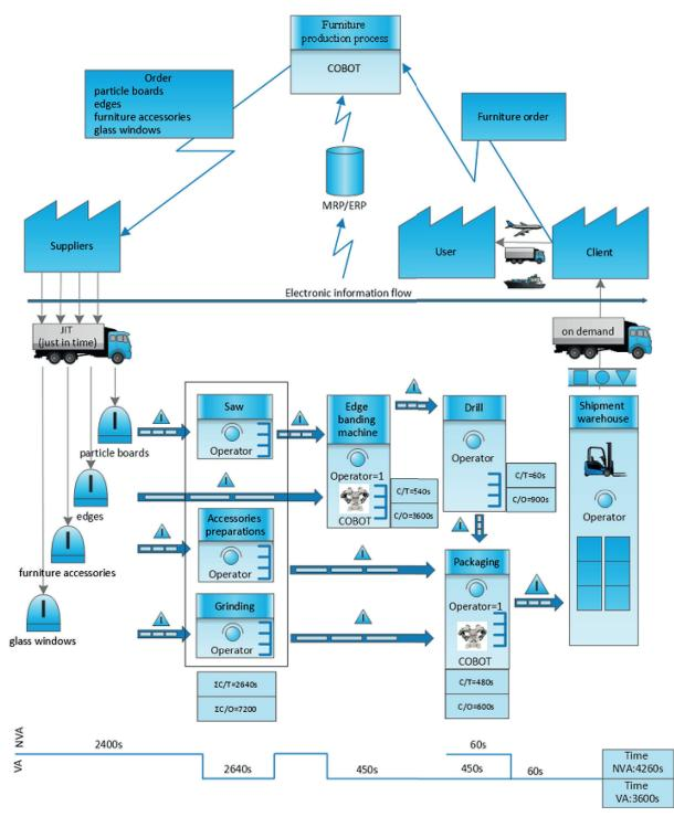
Figure 5. Value stream map of the furniture production process – a cobot perspective
