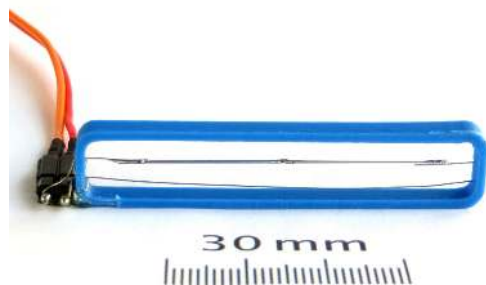
Figure 3. Sensor used for the measurement of the temperature of the air circulating inside COCAP. The sensing element (located in the centre of the blue 3-D-printed frame) is a miniature thermistor (1 mm × 0.5 mm × 0.5 mm). Two 23 mm long pieces of 0.5 mm wire are soldered to both sides of the thermistor. They conduct heat, facilitating the measurement of a temperature that is averaged across the air stream.
