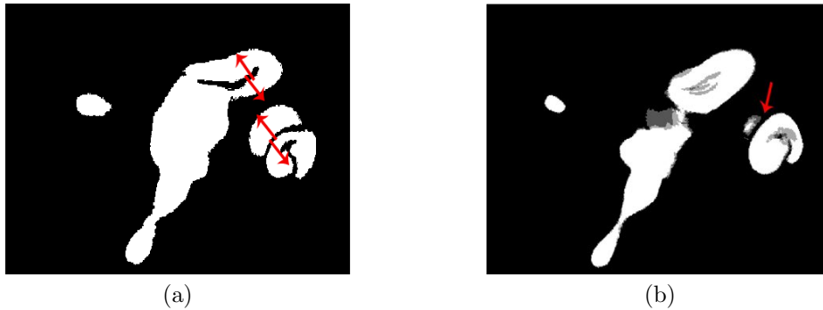
Figure 2. Leakage prevention. (a) Topology preservation where the red arrows indicate that the unit normal vectors of the corresponding points are pointing in opposite direction. Thus, the contour is not allowed to evolve along these points. (b) Error control map prevents leakage, for example the red arrow shows that the contour in this area will not evolve and merge with the other turn of the cochlea and in case there was leakage in the error map in this area, both turns would not merge either, due to the topology preservation method.
