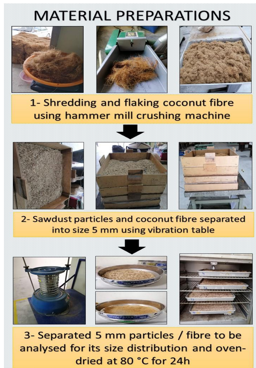
Figure 2. Sawdust Particle and Coconut Fibre Preparations.
