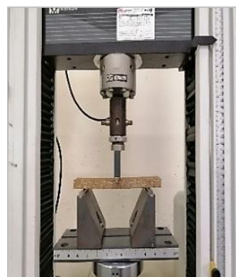
Figure 10. Mechanical properties for each particleboard determined by (a) the specimen tested using Universal Testing Machine; (b) after failure, the graph and value for Modulus of Elasticity (MOE) and Modulus of Rupture (MOR) appeared on screen.
