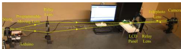
Figure 10: Our prototype and its light path. We use the moving lens and LCD panel for focal stack modulation, and the relay lens and telephoto lens are used to match the field-of-views.
