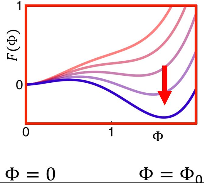
Near field imaging has revealed the discrete, 1<sup>st</sup> order nature of the phase transition in NdNiO<sub>3</sub>
