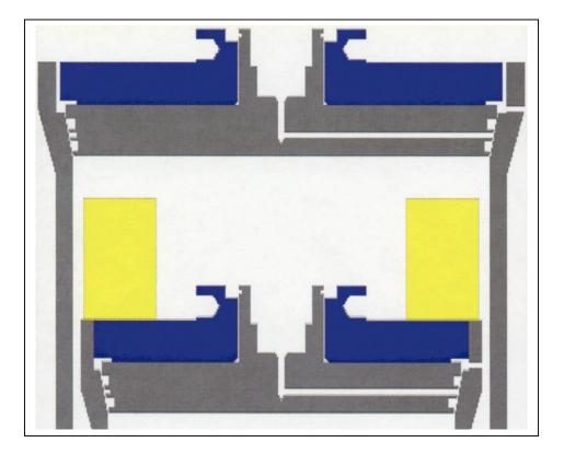
The example above shows the upper portion of the inner and outer containment vessels in the 9975 Type B shipping container. This COG model was translated from a Pro-E<sup>10</sup> model developed by the packaging designers at the Savannah River Site. This model makes extensive use of the REVOLUTION (closed surface) card in COG.
