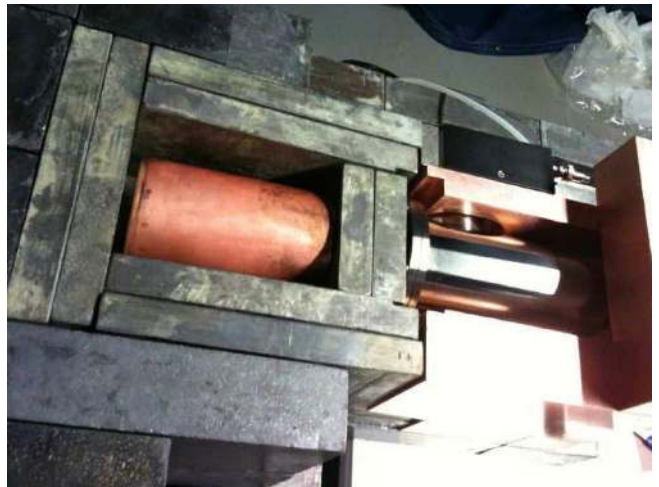
FIG. 1. Partially disassembled shield of the CoGeNT detector at SUL, showing the cylindrical OFHC end cap and innermost 5 cm of ancient 0.02 \text{ Bq } ^{210}\text{Pb}/\text{kg} lead, characteristically oxidized following etching. The preamplifier is visible at the top right (black box). A minimum of 7 cm of lead thickness shields the detector from the naturally occurring radioactivity in the preamplifier's electronic components.
