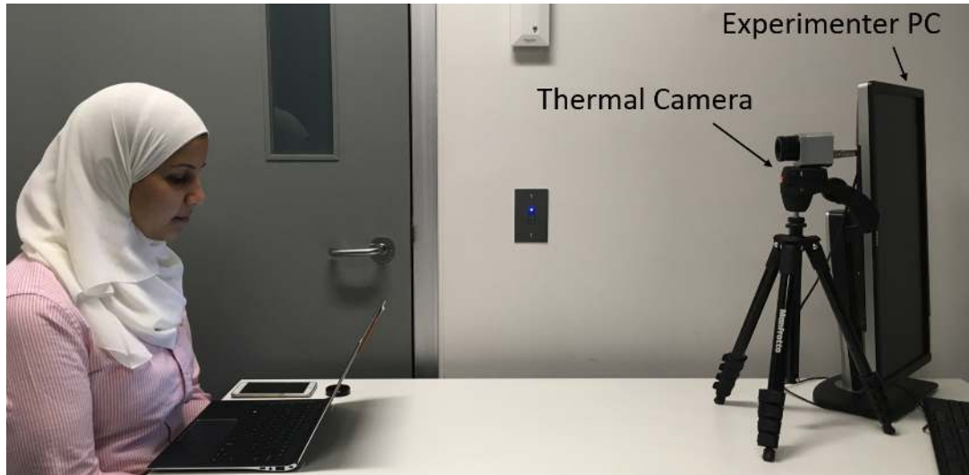
Fig. 1. Study setup consisting of thermal camera facing the participant while performing the reading task.
