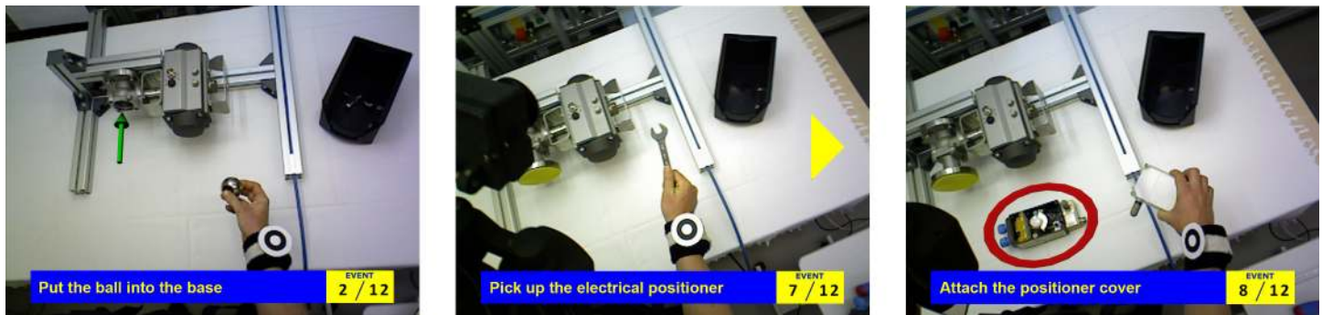
Fig 10. Overlays visualized in the HMD. Textual descriptions provide information on the current action and its position in the overall workflow. Relevant directions are indicated by 3D arrows. Relevant objects are highlighted by red circles (regions of interest). The yellow arrow at the right margin of the middle picture directs the attention of the user to the relevant part of the workspace, where in this case the electrical positioner is located and highlighted by a region of interest.
