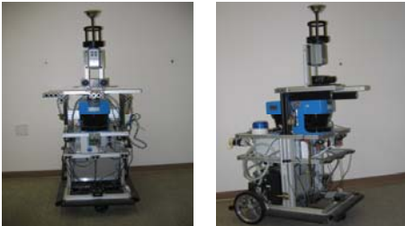
Fig. 4 The robot platform that was used for the experiments. The encoders, stereo vision system and laser scanners were used for this work.
