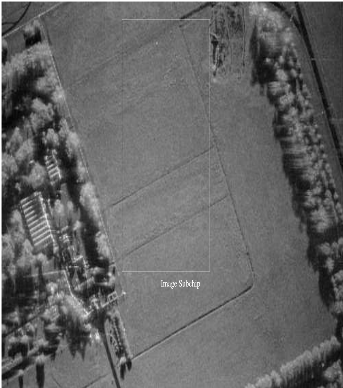
Figure 47: Intensity SAR image generated from the primary pass imaging collection processed to a resolution of 0.52 m (range) by 0.150 m (azimuth) with a Hamming window applied.
