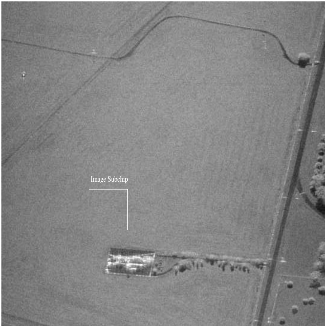
Figure 36: Intensity SAR image generated from the primary pass collection processed to a 3 dB resolution of 0.61 m (range) by 0.15 m (azimuth) with a Hamming window applied. Also shown is the image subchip selected for further processing and change detection analysis.
