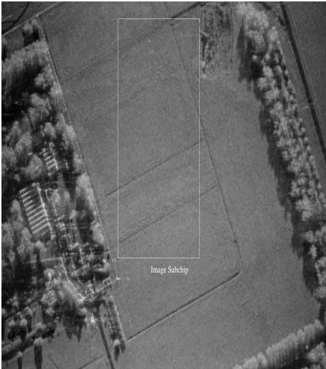
Figure 48: Intensity SAR image generated from the repeat pass imaging collection processed to a resolution of 0.52 m (range) by 0.150 m (azimuth) with a Hamming window applied.
