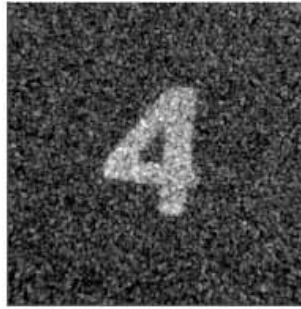
Figure 9. Ghost image of the number 4, retrieved from the correlation function after averaging over 30 000 shots.
