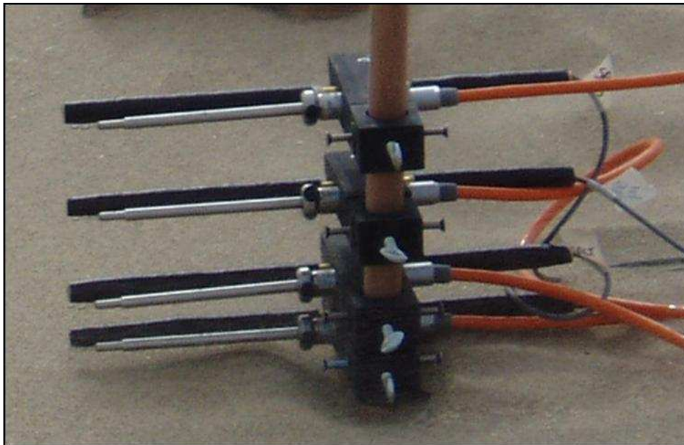
Fig. 3-10. Thermal anemometers (silver) and miniphones (black) mounted on an instrument tower at 0.02, 0.06, 0.12, and 0.20 m above the bed. A portion of a sand trap can be seen on the top of the photograph. This photograph was taken during a Configuration A run. Only the bottom TA-MIC pairs are used in this research.
