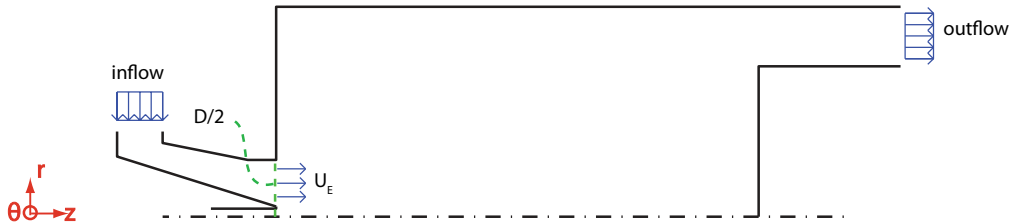
Figure 1: Illustration of the flow geometry. A cross-section in the axial-radial plane (constant azimuthal angle), showing the inflow (swirler inlet) and the outflow. The nondimensional scales are shown: swirler outer diameter ( D ), and the exit velocity from the swirler ( U_E ). The coordinate system is also defined: the origin is at the centerline at the swirler exit location. The relative dimensions of the geometry are the same as in the numerical simulation, except that the numerical domain is longer in the downstream direction.
