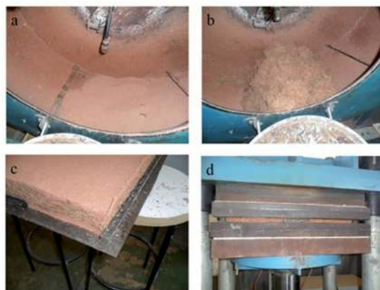
Figure 1: MDP production. (a) Adhesive application to smaller particles. (b) Adhesive application to bigger particles plus fibers. (c) Particle mattress after the pre-pressing. (d) Particle mattress during the hot press.
