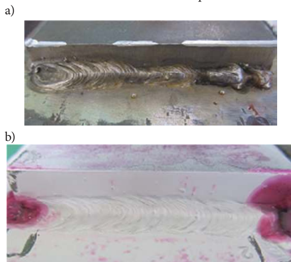
Fig. 3. Results of non-destructive testing of S460N steel joints; a) VT, the specimen W2, the first-laid weld: incompletely filled groove, incomplete fusion; b) PT, the specimen W1 : no imperfections.
