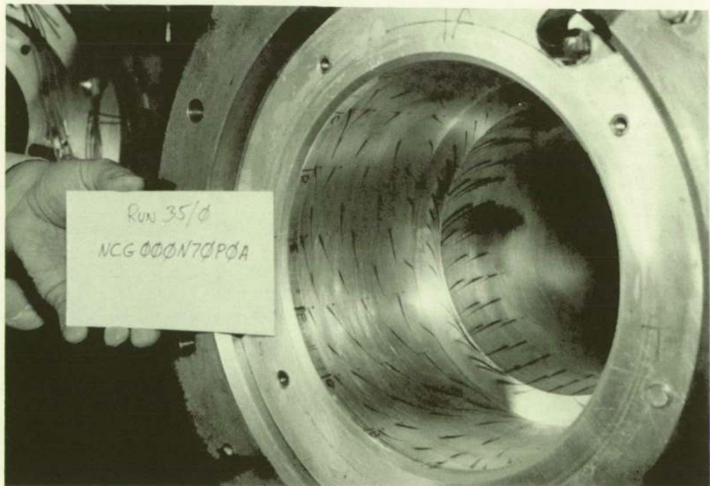
Fig 3. Oil Flow Pattern in Lower Half of Propellant Grain, Aft End; Propellant Grain = 0 Sec, Nozzle Angle = 7^{\circ}
