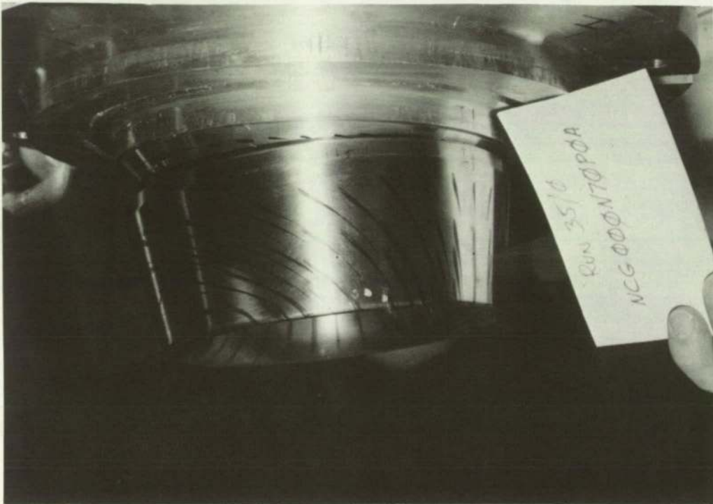
Fig 4. Oil Flow Pattern on Nozzle Nose; Propellant Grain = 0 Sec, Nozzle Angle = 7^{\circ}
