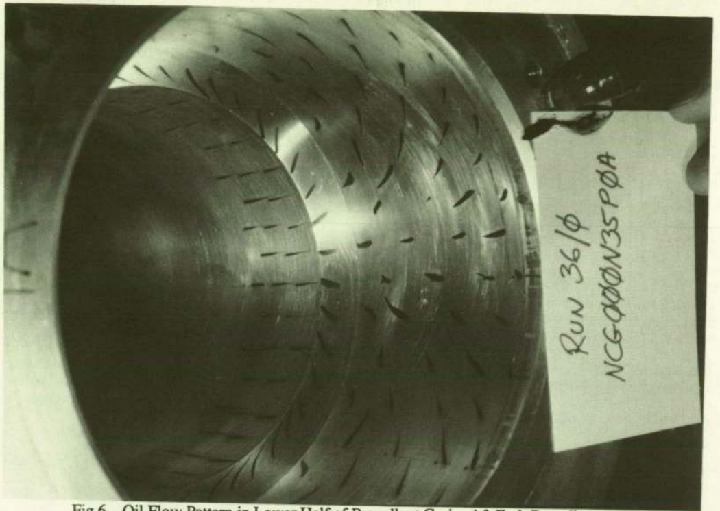
Fig 6. Oil Flow Pattern in Lower Half of Propellant Grain, Aft End; Propellant Grain = 0 Sec, Nozzle Angle = 3.5^\circ
