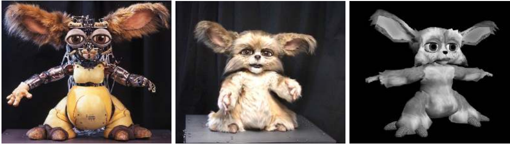
Figure 5. “Leonardo”, the expressive humanoid robot used in this study. The left picture shows the robotic structure, the center picture shows the robot when cosmetically finished, the right shows a simulated version of the robot.
