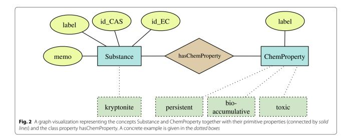
For instance, the identities EC and CAS number, a textual memo, and a name label are connected with the class *Substance*. Also the class *ChemProperty* has a name label. The class relation *hasChemProperty* connects classes by a diamond. Example instances are given below in dotted lines: For demonstration purposes, we use as example the fantasy substance *Kryptonite*, for which we define persistent, bioaccumulative, and toxic properties.
