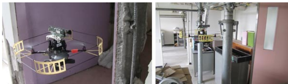
Figure 5. The aerial robot flies through cluttered regions of the environment that are inaccessible to the ground robot and builds a 3D map that will be merged with the maps made by the ground robot.
