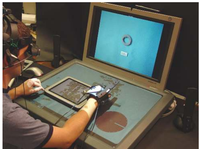
Figure 7. Handheld widget is used on the Diamond-Touch table to show high-resolution version of the portion of the 2D map that it covers.
