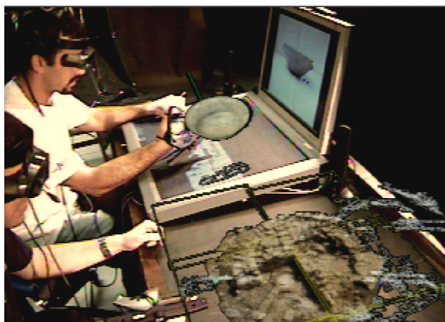
Figure 1. Two users simultaneously collaborate in VITA. While one user is inspecting the 3D virtual model of the ceramic vessel above the table comparing it with the high resolution image on the screen, the second user is looking at the 3D miniature terrain model next to the table. All AR images in this paper are captured through a live tracked video see-through display.
