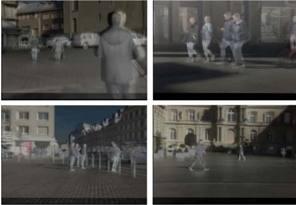
Fig. 2. Examples of synchronized pairs of visible and far-infrared images using the infinite homography registration. People close to the stereoscopic system are not well synchronized, people far from it are well synchronized.
