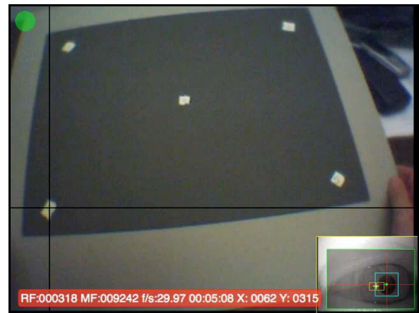
Figure 4. Static point array method for conducting a five-point calibration on mobile eye-trackers. In this video still from research conducted our laboratory, observers who were tracked while assembling a small device viewed five calibration stickers affixed to a hand-held board.
