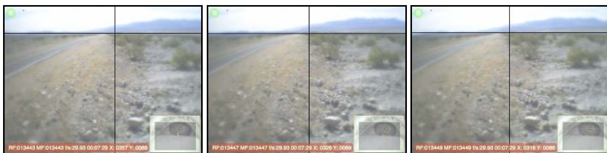
Figure 15. Effect of head motion compensation during slow head rotation. Shown above are median frames from three separate fixations that were detected when head motion compensation was not applied; with head motion compensation, these were combined into a single fixation.
