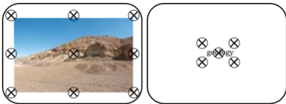
Figure 3. Sample calibration points for computer-based eye-tracking studies. Calibration points extend just beyond the stimulus borders, covering the full screen in experiments with large stimuli (nine-point array at left) and a reduced area for smaller stimuli (five-point array at right).
