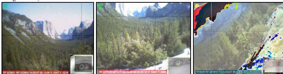
Figure 16. Lack of correspondence between fixated object and its location in the scene video. In each of the above frames, the observer is fixating the same feature (a hanging valley), but head movements and the different positions of each observers cause the feature's location in the scene video to vary.
