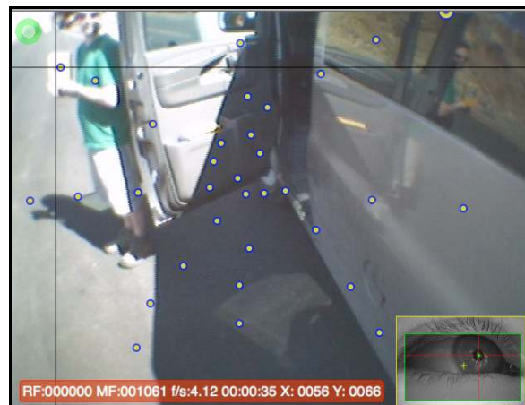
Figure 6. Head tick calibration method. The observer is looking at a stationary target held by a partner, and the dots indicate all positions the observer paused for a head tick.
