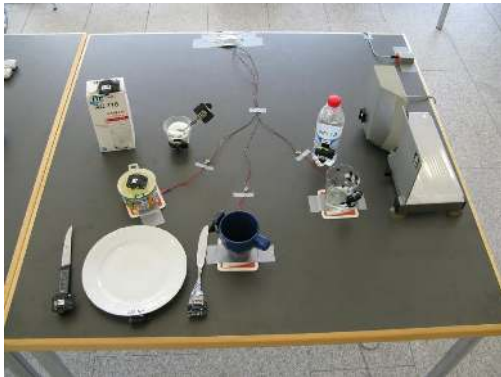
Fig. 5. The objects are instrumented with an acceleration and rate of turn sensor node. Visible are also the bread slicer (right), an XSense measuring table vibration (far right), and pressure sensors under some of the tableware. Not visible: the identically instrumented bread and salami.
