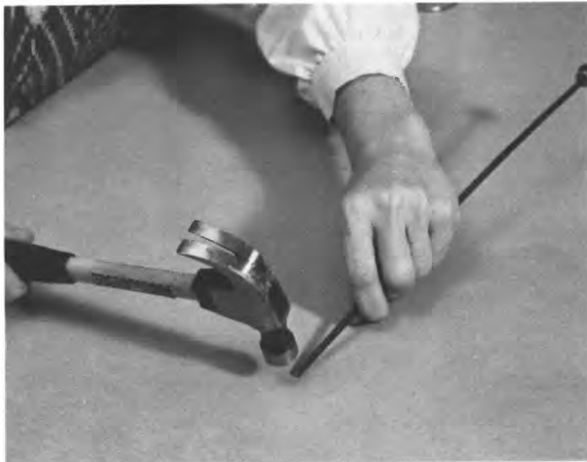
Figure 15. - Opening end of extractor spoon with hammer when the extractor jaws against the core before complete insertion.
