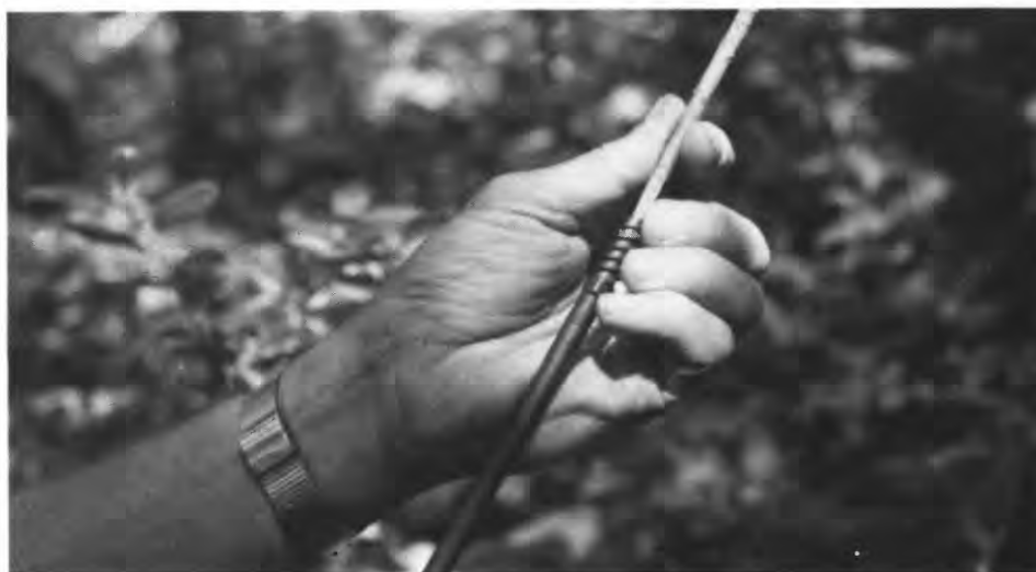
Figure 20. -Removing a core plug using a wooden peg. The first consideration is to avoid damaging the cutting edge of the bit.
