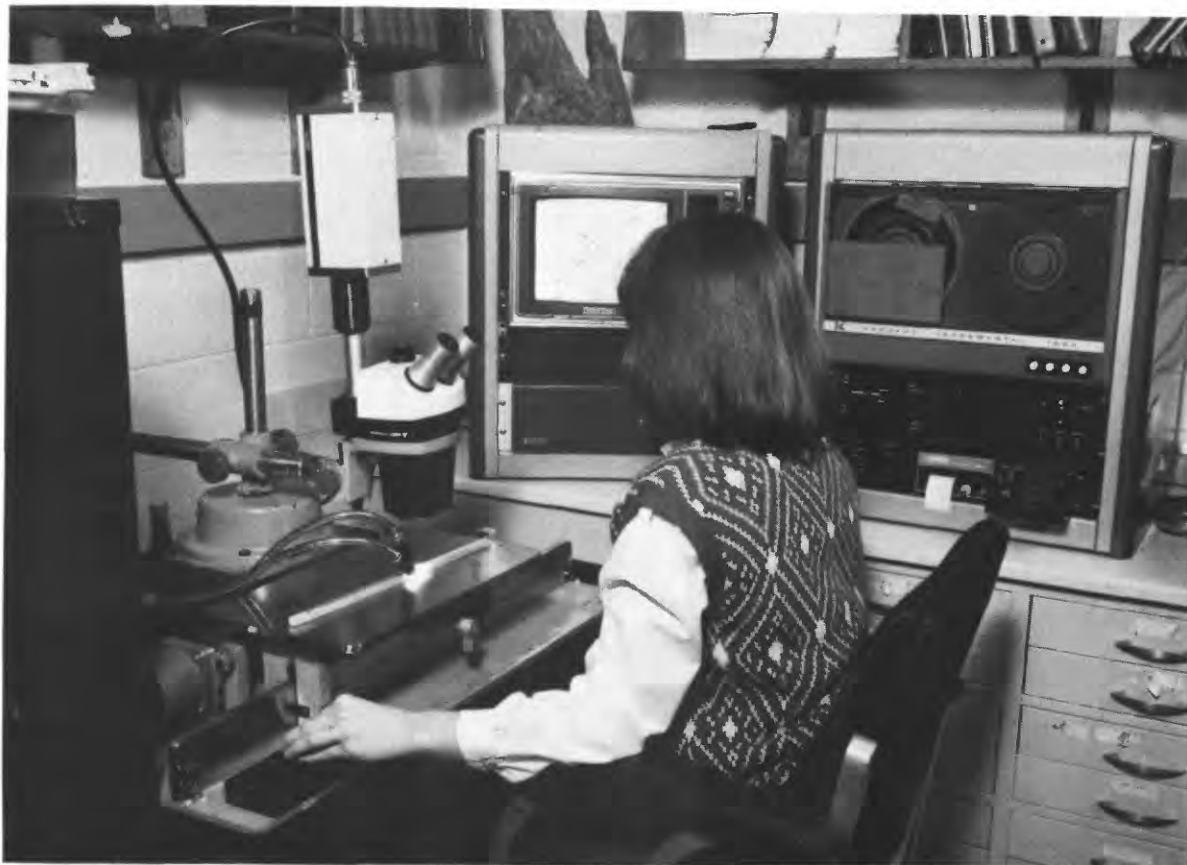
Figure 42. -Automated equipment for measuring ring widths.
