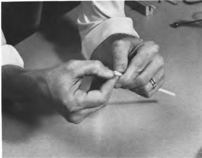
Figure 26. - Folding ends of paper straw. Make four creases with a thumbnail, and then fold in.
