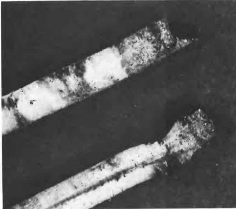
Figure 10. -A correctly shaped, straight core, and a core with bends near the outside resulting from not maintaining a steady borer.
