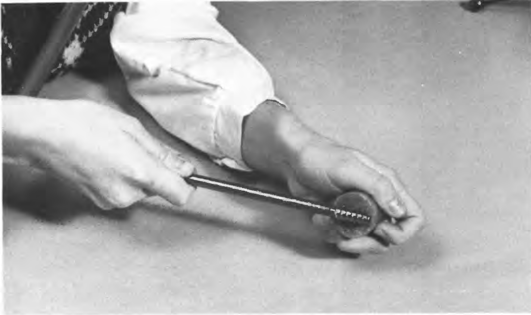
Figure 8. - Beeswax is applied to lubricate the borer bit threads.
