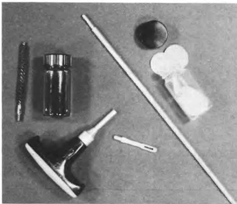
Figure 5. -Cleaning kit modified from a commercial kit for .22 caliber rifles. The swatch holder has been filed to easily fit the cutting-edge end of the borer bit, and the rod attached to the handle has been shortened.
