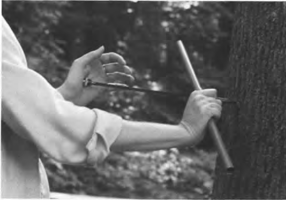
Figure 12. -Insert the extractor in a steady, continuous motion.
