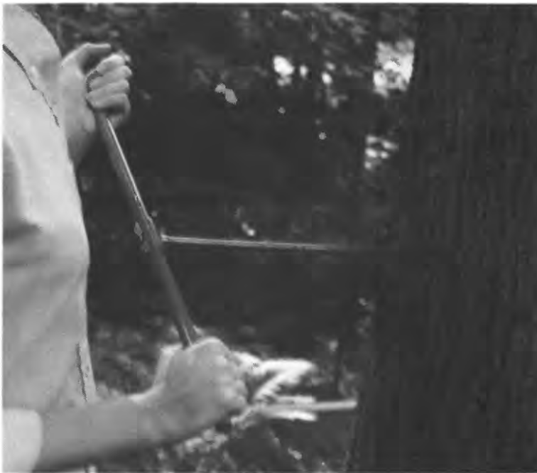
Figure 11. -Pressure need not be applied to push the borer into the wood after the bit threads have engaged the wood.
