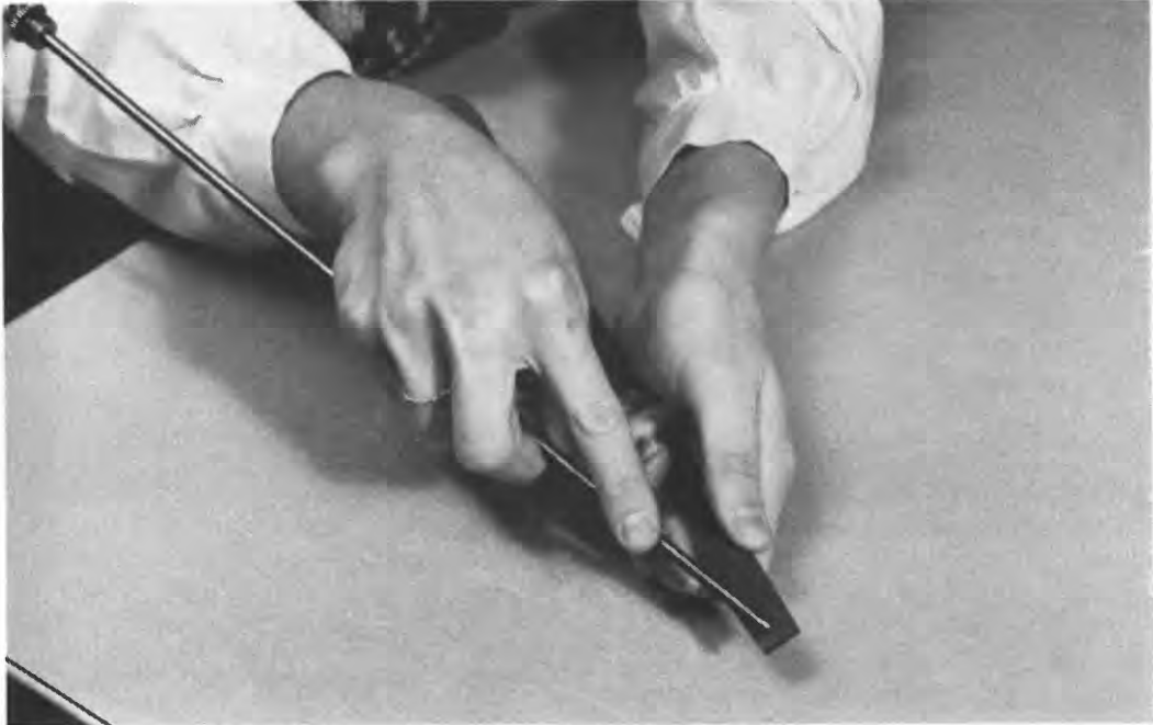
Figure 14. - Filing inside surface of extractor spoon to allow the extractor to slide more easily between the core and bit tube.
