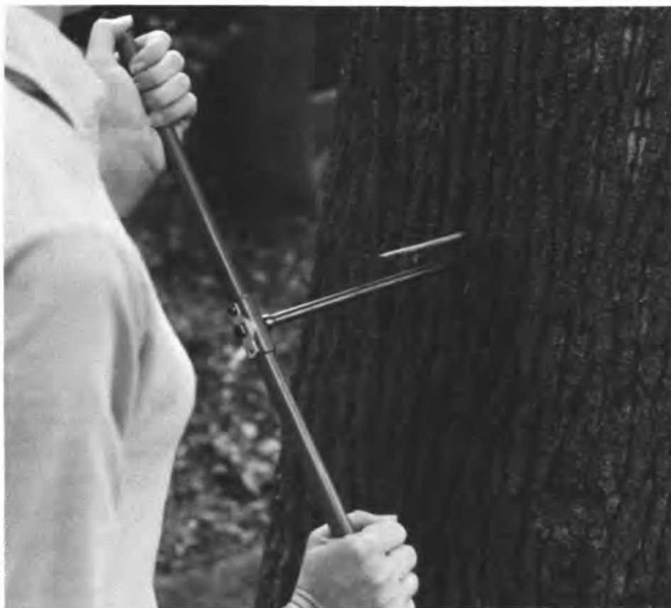
Figure 22. -Orienting increment borer parallel to, and at correct direction and distance from, first core hole in order to obtain botanical center with second core.
