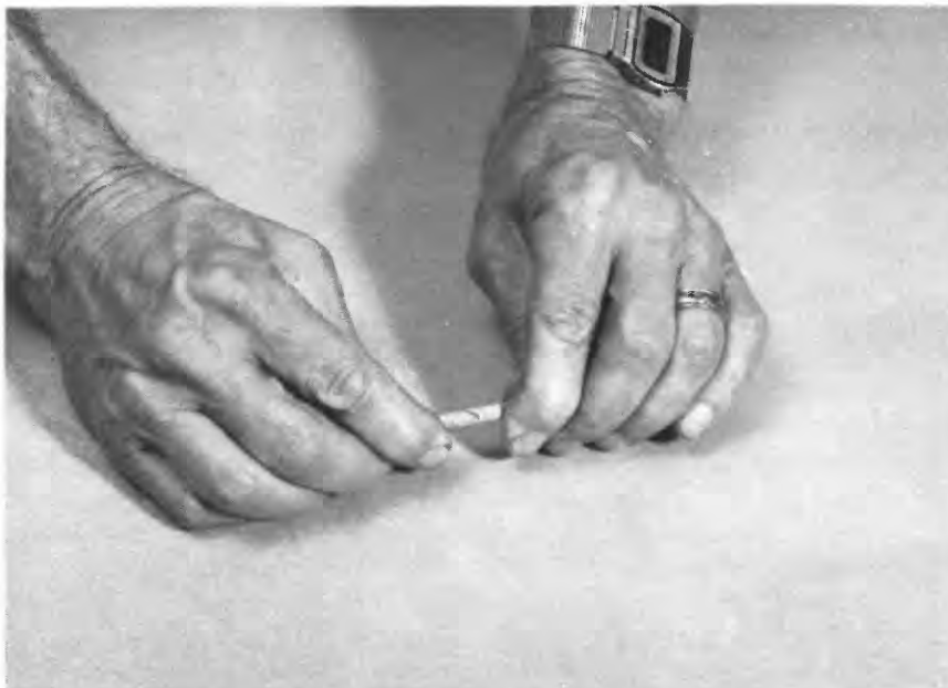
Figure 29. - Breaking apart a partially cut core after a diagonal cut has been made about half way through the core.
