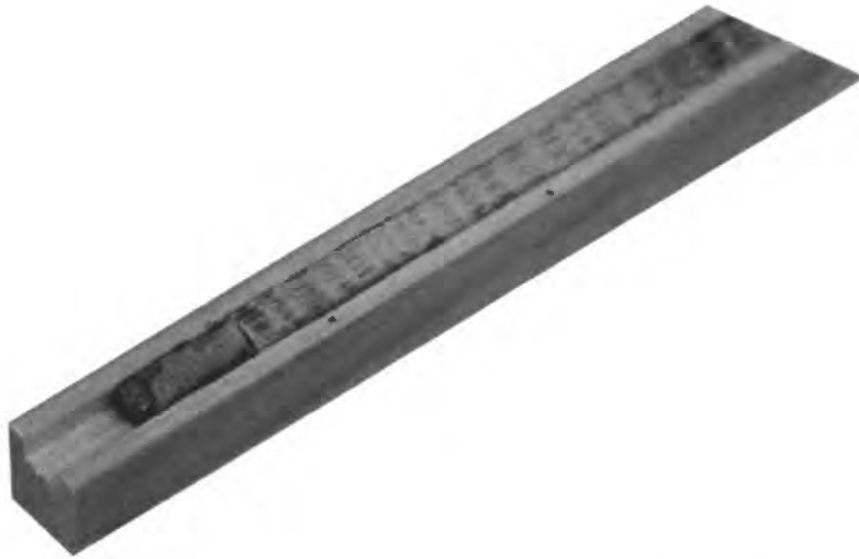
Figure 31. -Core permanently mounted in block.
