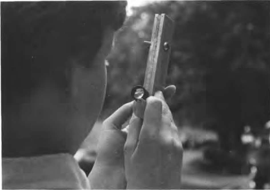
Figure 25. -Examining shaved core in the field with core clamp and hand lens.
