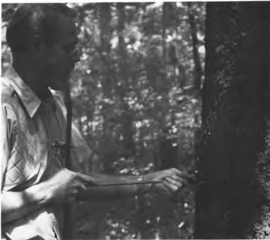
Figure 9. - Start the increment borer by a combination of pushing and turning with one hand while steadying the bit with the other hand.
