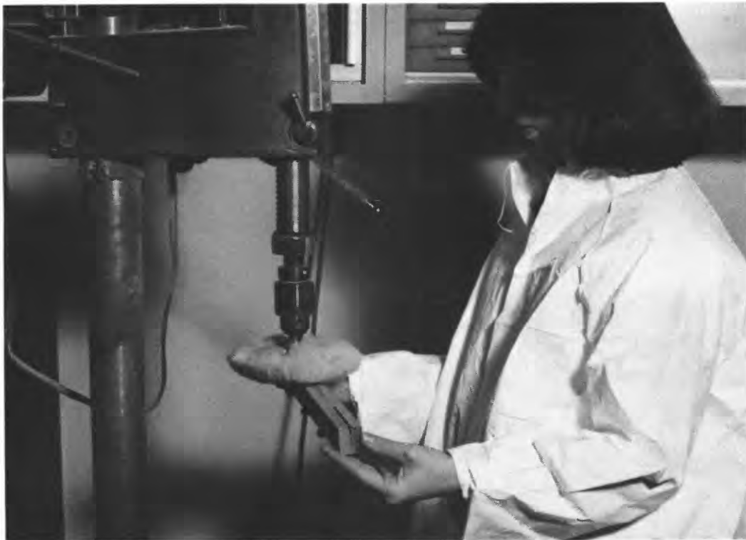
Figure 36. -Using a lamb's wool buffing pad to polish and dust a surfaced increment core.
