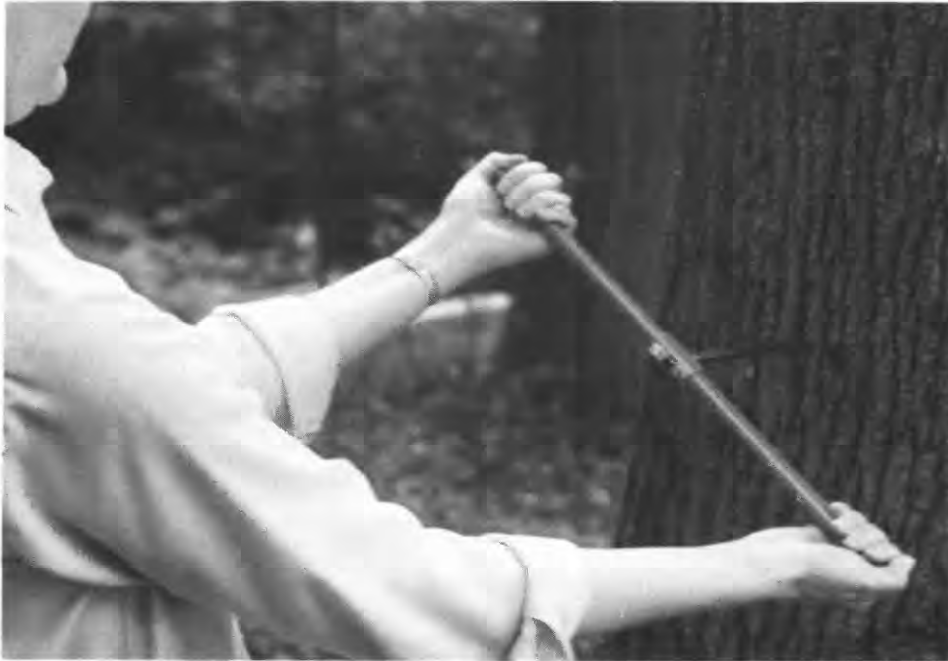
Figure 18. -Using the jerk-and-turn method to remove a stuck borer. This procedure usually engages the threads, after which the borer can be removed in the normal manner.
