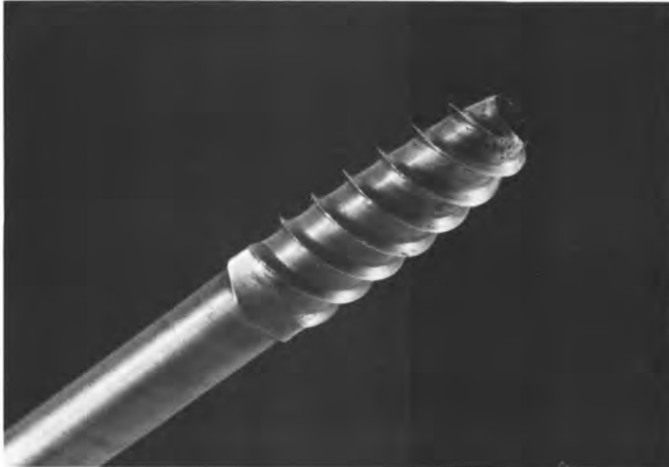
Figure 6. -End of increment borer bits from which pieces have broken away as a result of metal fatigue.
