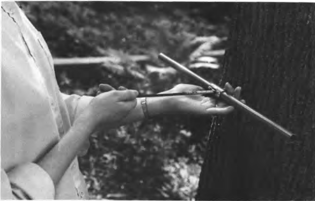
Figure 17. -Removing core. Use one hand to steady the extractor and catch any loose core pieces that might fall out of the spoon.
