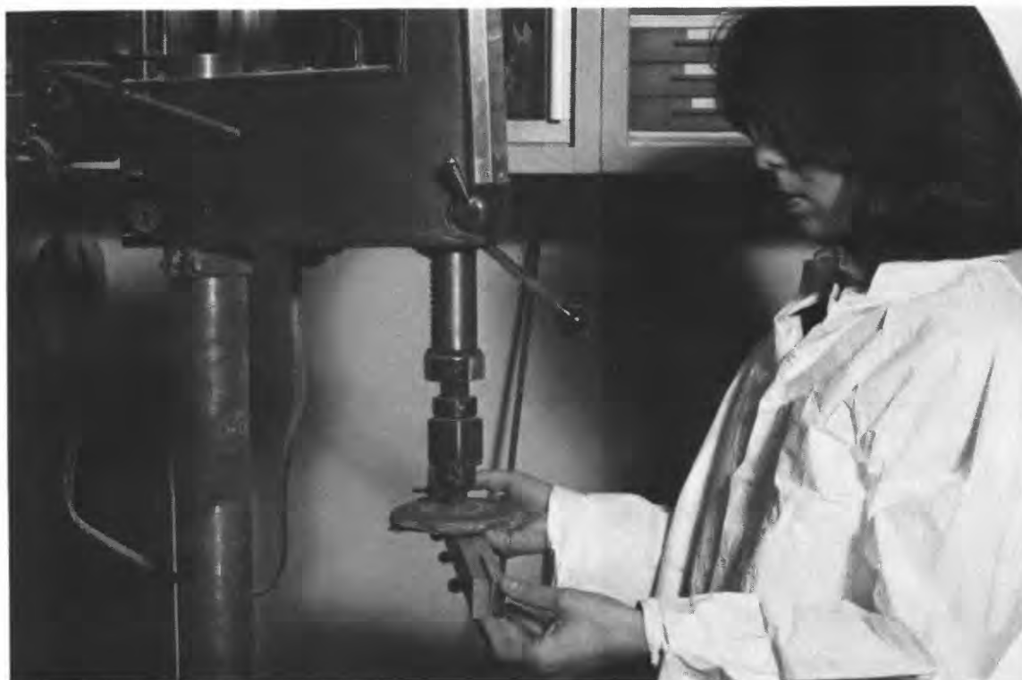
Figure 35. -Preparing a sanded surface on an increment core using a sanding disc mounted on a drill press.
