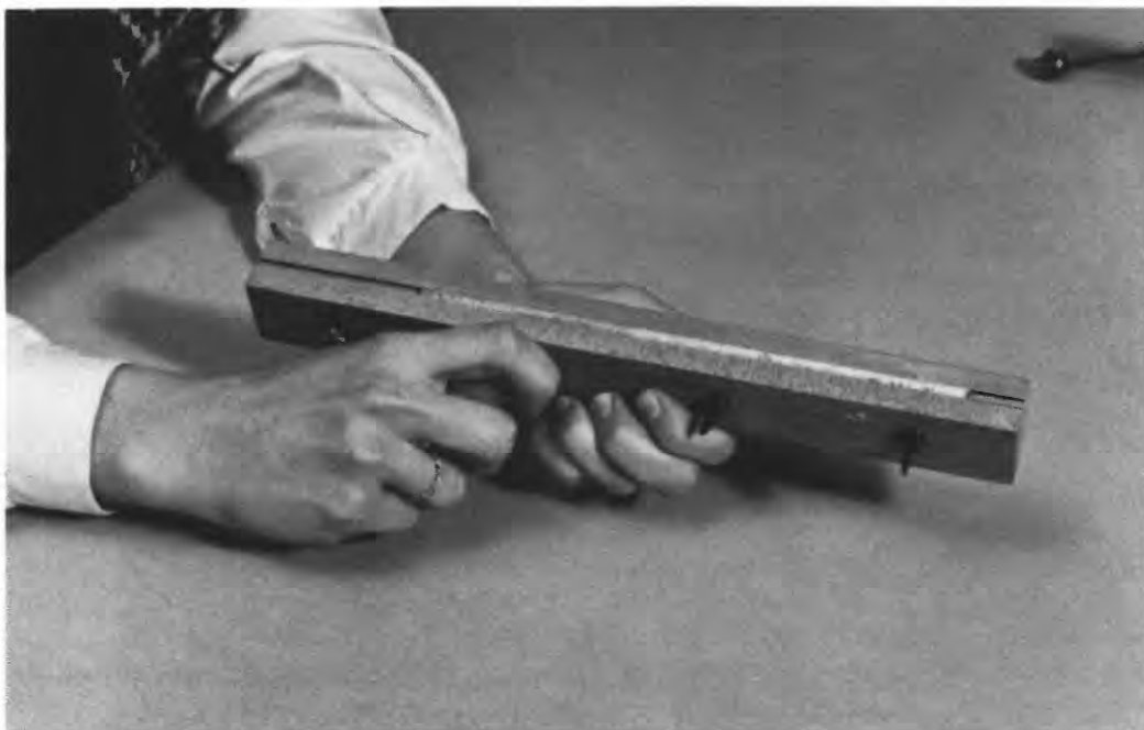
Figure 23. -Core clamp used to hold core during surfacing, crossdating, and measuring.
