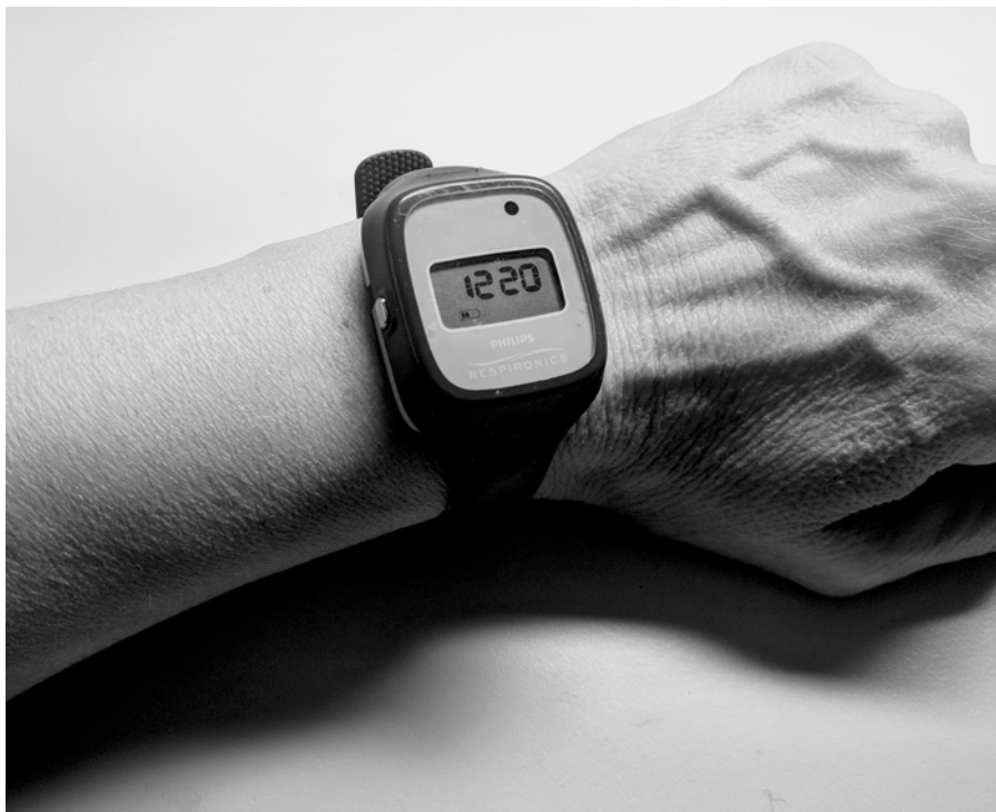
Figure 2: The activity monitor/accelerometer device worn on the wrist of the non-dominant hand. Please click here to view a larger version of this figure.
