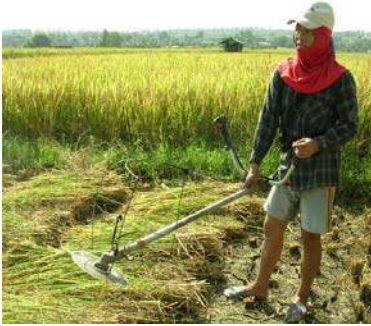
Figure 4.6. Modified weed slasher for harvest
