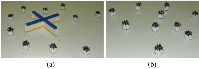
Figure 6: Preliminary experiments with 10 microrobots; (a) Collective perception; (b) Building a "communication street".
