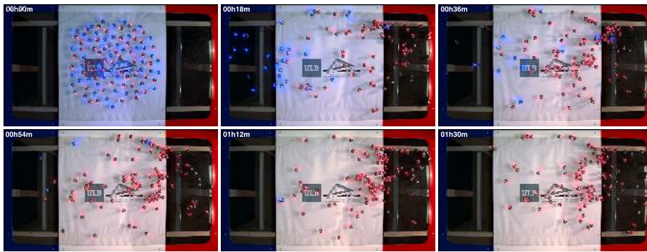
Fig. 4 The figure shows a series of screen-shots taken from one experiment with a swarm of 100 Kilobots. The screen-shots are taken every 18 minutes of execution.
