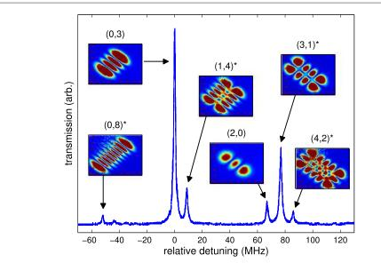
**Figure 3.** Transverse cavity modes. The solid curve shows a number of cavity transmission resonances (without atoms), and insets show the corresponding spatial profiles as imaged onto a camera. The  $45^{\circ}$  tilt of the patterns reflects the orientation of the cavity plane ( $\chi_{2}$ ). The modes are labelled according to transverse indices (*m*, *n*), with asterisks denoting a longitudinal index *q* which is one less than that of the (0, 3) mode which is taken as reference.
