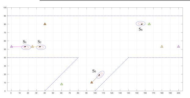
Figure 15. Verification of collision avoidance in a multi-ship situation.
