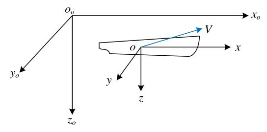
Figure 4. Ship-maneuverability motion coordinate system.
