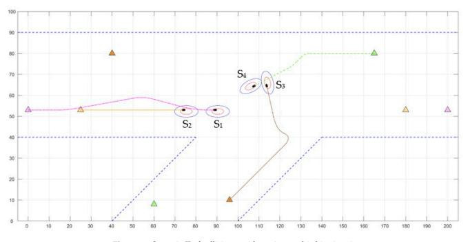
Figure 17. Scenario II of collision avoidance in a multi-ship situation.
