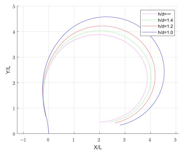
Figure 6. Turning test trajectory.
