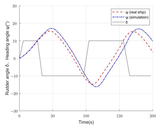
**Figure 7.** Right  $10^{\circ}/10^{\circ}$  Z-type maneuver test.
