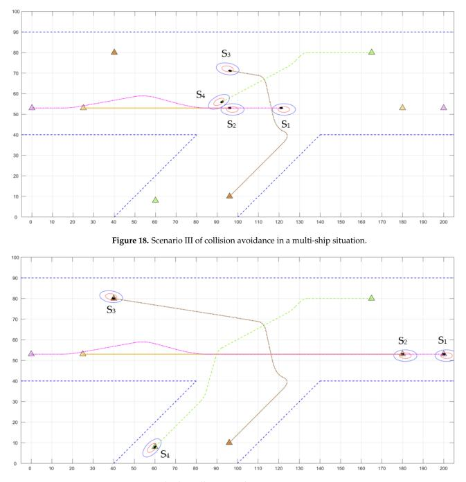
Figure 19. Multi-ship collision-avoidance trajectory.
