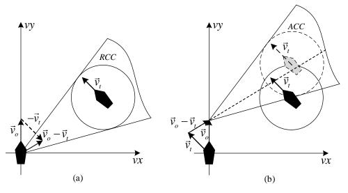
Figure 1. Velocity obstacle algorithm: (a) RCC and (b) ACC.
