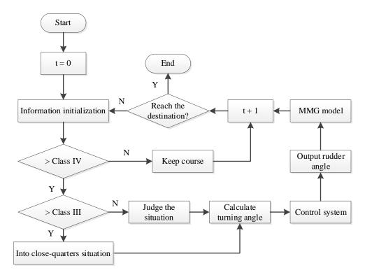
Figure 13. Flow chart the of collision-avoidance decision system.
