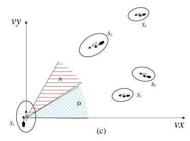
Figure 11. Combination of velocity obstacle cones: (a) determination of common tangents, (b) construction of VO cones, and (c) merging VO cones.
