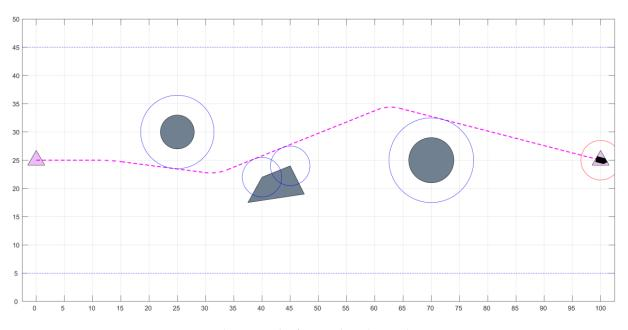
Figure 14. Simulation result of static-obstacle avoidance.
