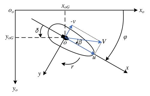
Figure 5. The horizontal view of the ship's maneuverability motion coordinate system.
