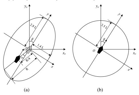
Figure 3. Inland-ship domain for: (a) dynamic obstacles, (b) static obstacles.
