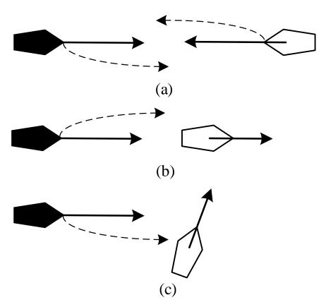
Figure 2. Inland-ship encounter situations: (a) head-on, (b) overtaking, and (c) crossing.
