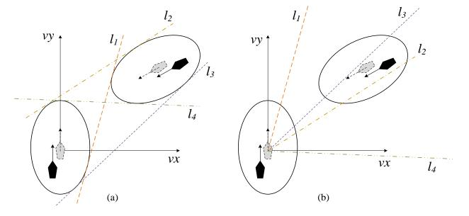
**Figure 10.** Avoidance in the elliptical ship domain: (**a**) determination of common tangents, (**b**) construction of VO cones.
