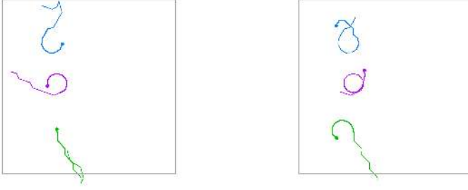
Fig. 4 Trajectories of the three UAVs doing maneuver to avoid collision.
