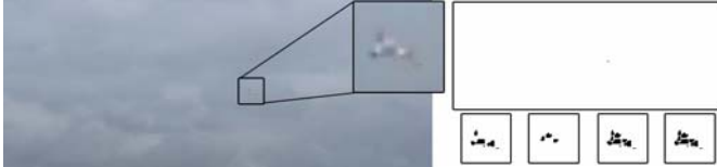
Fig. 9. Example of the situation with middle contrast clouds: on the left the original image with the enlarged aircraft; on the upper right the result of first adaptive threshold, on bottom right from left to the right the darker pixels, brighter pixels, OR operation and the segmented aircraft
