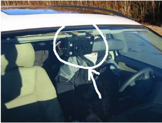
Figure 8.5: The laser radar installed behind the windshield of the demonstrator vehicle.
