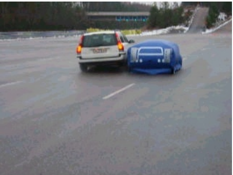
(c) The maneuver is sufficient to avoid the obstacle with the smallest possible margin.
