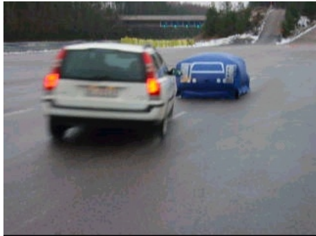
(b) At the last moment the driver makes an evasive steering maneuver.
