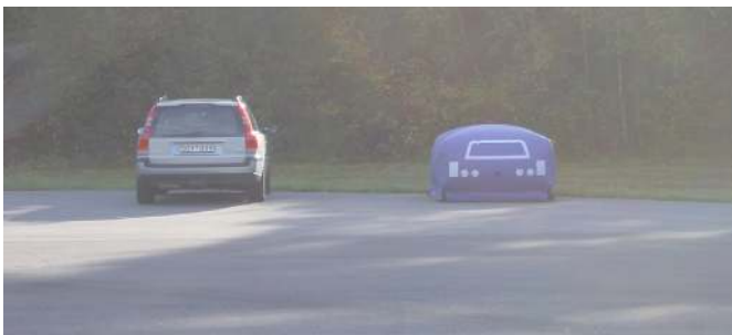
Figure 8.8: In measuring the radar response from the back of a Volvo V70 and from the inflatable car, it was found that the radar echo was as strong from the inflatable car as from the Volvo in this particular set up.
