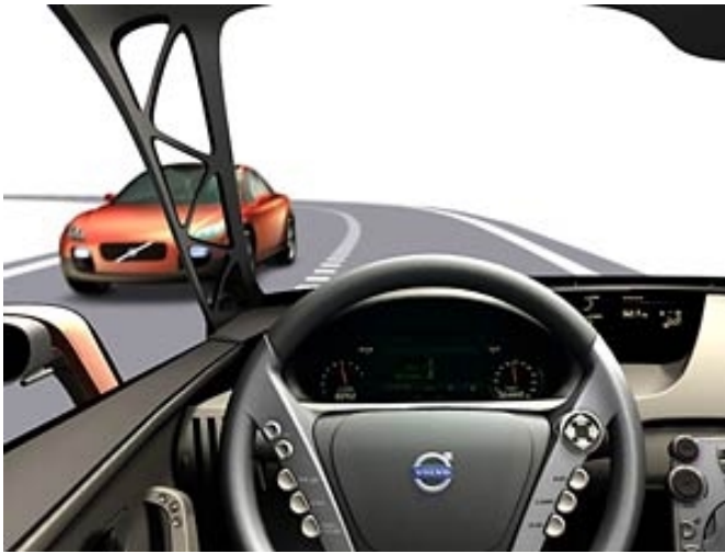
Figure 2.2: One safety technology, aimed to improve the drivers perception, presented in the Volvo safety concept car was a see-through A-pillar.
