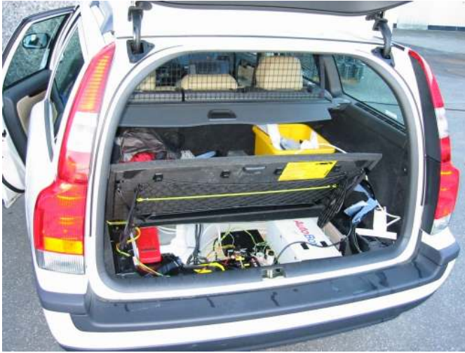
Figure 8.2: The dSPACE unit is installed under the floor of the luggage compartment
