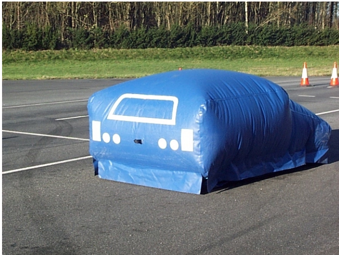
Figure 8.3: Inflatable car used for collision test, maximum collision speeds 70 km/h.
