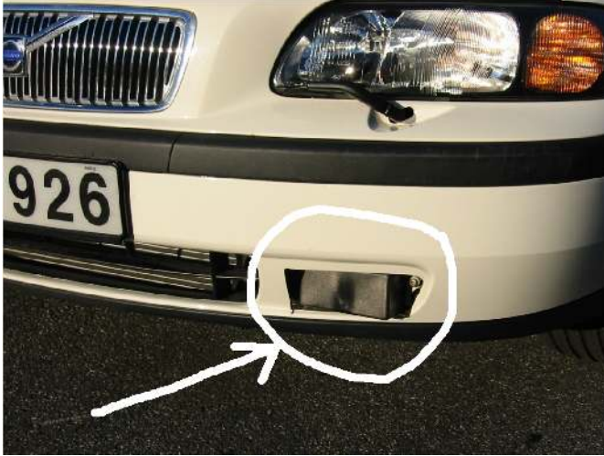
Figure 8.4: The mm-radar installed in the front bumper of the vehicle.
