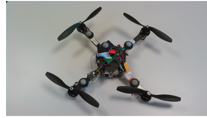
Fig. 4. The AscTec Hummingbird used in the experiments.
