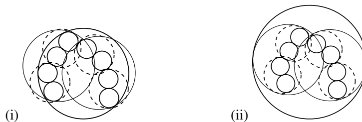
Figure 2. Wrapped (left) and layered (right) sphere hierarchies. The base beads are black. Notice that each cage in the wrapped hierarchy is supported by 2 or 3 beads.
