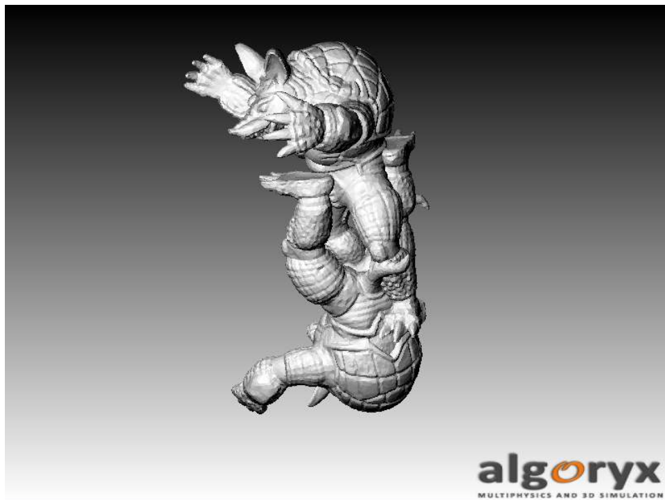
Figure 6.1: An example of a test scene with two armadillo objects colliding. These two objects are armadillo_3 objects, each consisting of 27 674 triangles.
