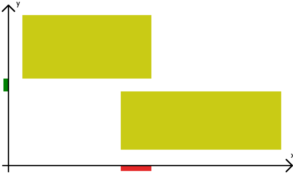
Figure 3.2: Example of two AABBs in intersection test in two dimensions. As can be seen, they are separated on one axis, which means the two boxes are not intersecting.
