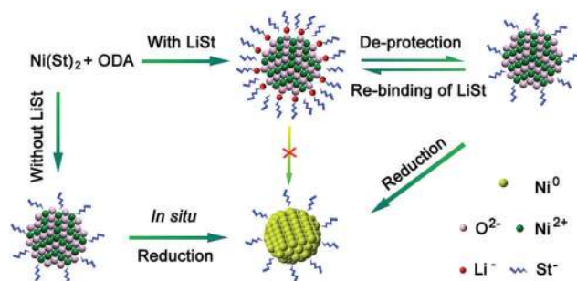
Fig. 6 Synthesis of colloidal NiO nanocrystals with LiSt as the protecting ligand. Abbreviations: ODA, 1-octadecanol; LiSt, lithium stearate; \text{Ni}(\text{St})_2 , nickel stearate. Figure reprinted with permission from ref. 25. Copyright 2014 American Chemical Society.
