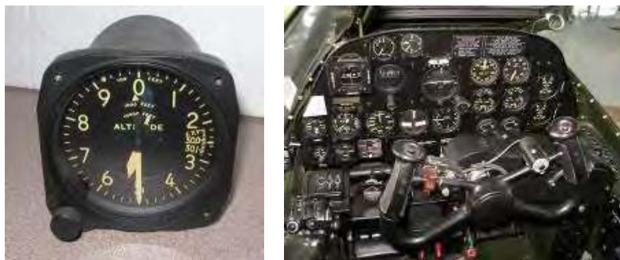
Figure 12. WWII era display with UV light illuminated indicia (left) and the displays installed in a P-38 cockpit (right).
