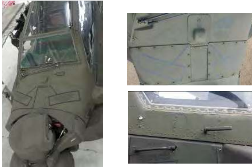
Figure 91. AH-64 Apache exterior markings for the emergency Canopy Jettison Handle (left), their blue-gray appearance following weathering (top, right), and the standard canopy handle (bottom, right).
