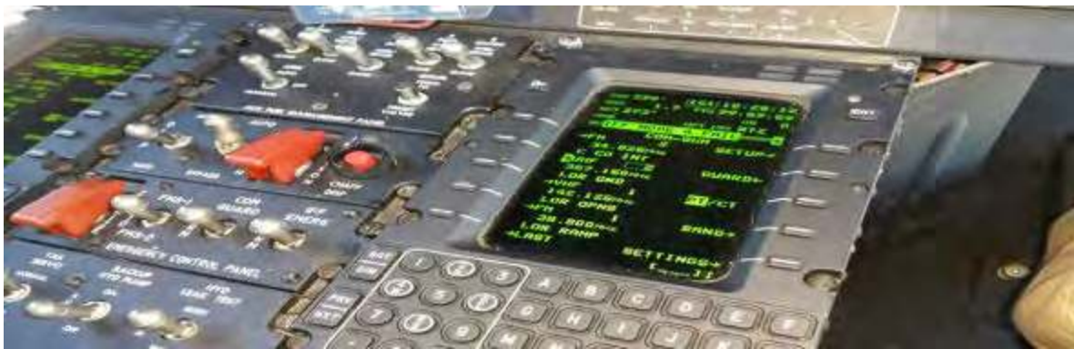
UH-60M red-orange colored switch guards on center console
