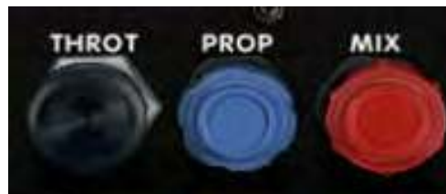
Figure 101. Color coding of engine controls in piston engine aircraft.
