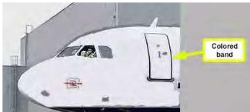
Figure 86. Example of colored band outlining side fuselage exit door on transport aircraft.
