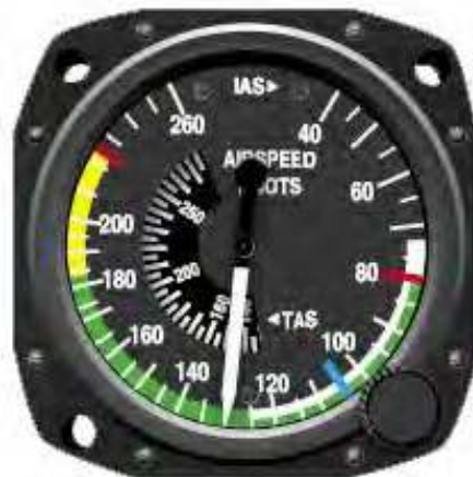
Figure 192. Example of multi-engine airspeed indicator (ASI) showing color arcs. The color codes are: White Arc, Green Arc, Yellow Arc, Red Radial Line, and Blue Radial Line.
