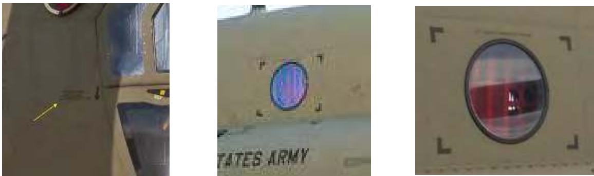
Figure 90. Exterior emergency markings on the CH-47F Chinook: jettison cockpit door (left); window right-angle corner markings (middle); and cut away rescue hatch (right).
