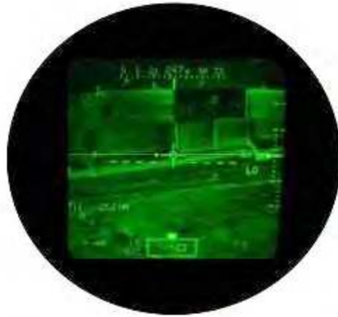
Figure 166. IHADSS yellow-green P-43 phosphor generated FLIR pilotage imagery with symbology overlay (enhanced photograph).
