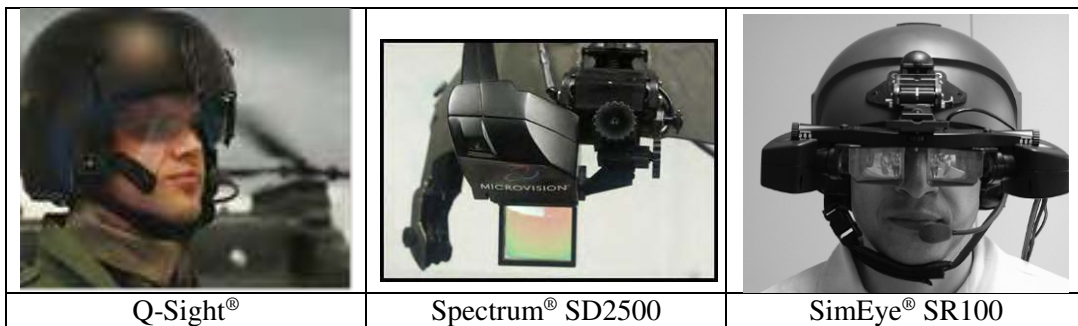
Figure 190. Examples of color HMDs: BAE Systems Q-Sight® (left); Microvision, Inc., Spectrum® SD2500 (middle); and Rockwell Collins, Inc., SimEye® SR100 (right).
