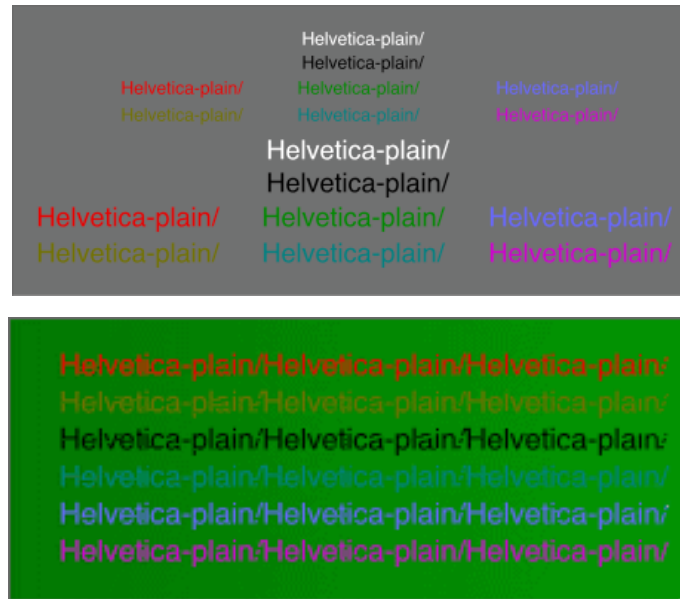
Figure 107. Examples of illegibility where a large hue difference exists, but luminance contrast is small (NASA Ames Research Center, 2000b).
