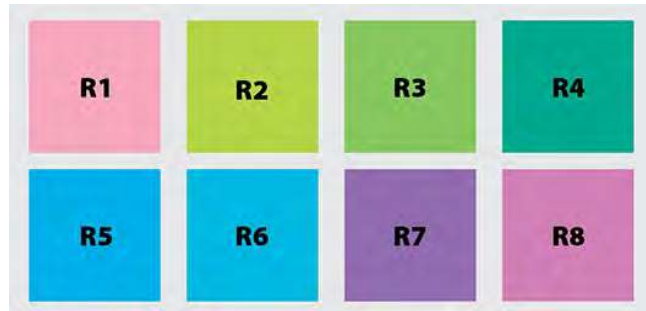
Figure 48. Test colors used in calculating CRI.
