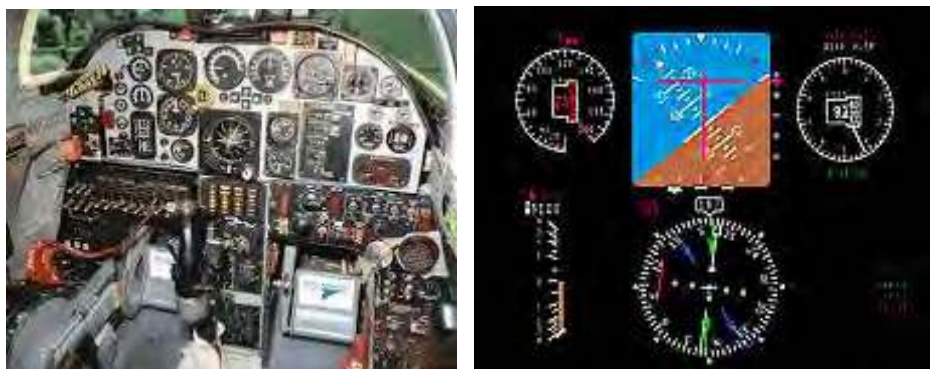
Figure 80. Use of white color to simulate previous generation cluster dials (left) on modern MFDs (right).
