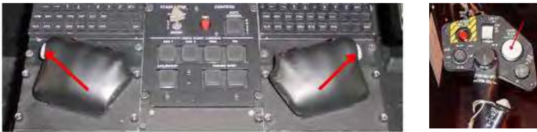
Figure 120. UH-60M DMS multi-function slew controllers (MFSC) positioned on each side of the center console (left) and a collective slew controller (CSC) mounted on each pilot's collective control (right). Red arrows denote the position of the white cursor slew buttons.
