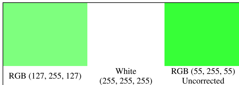
Figure 54. Example of uncorrected color gamma (right).
