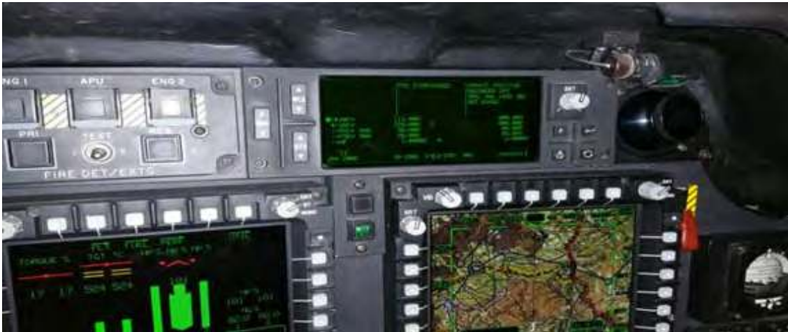
Pilot rear seat: Fire Detection/Extinguishing Panel (top, left) and Enhanced Up Front Display (communications) (top, right); dual MFDs (bottom, left and right)
