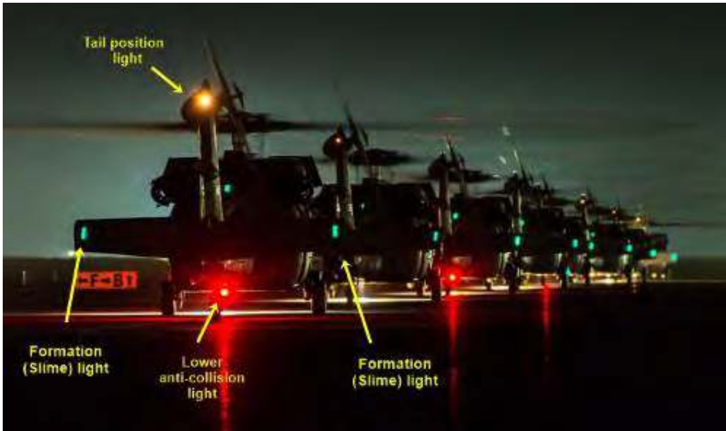
Figure 93. UH-60 Blackhawks lined up for formation flight, showing some position, formation, and anti-collision lights.
