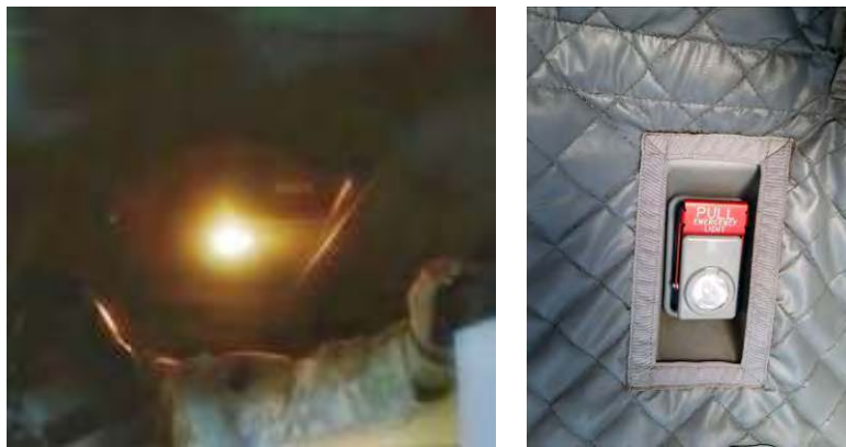
Figure 102. Example of CH-47F overhead dome light (left) and emergency light (right) in the cargo compartment.
