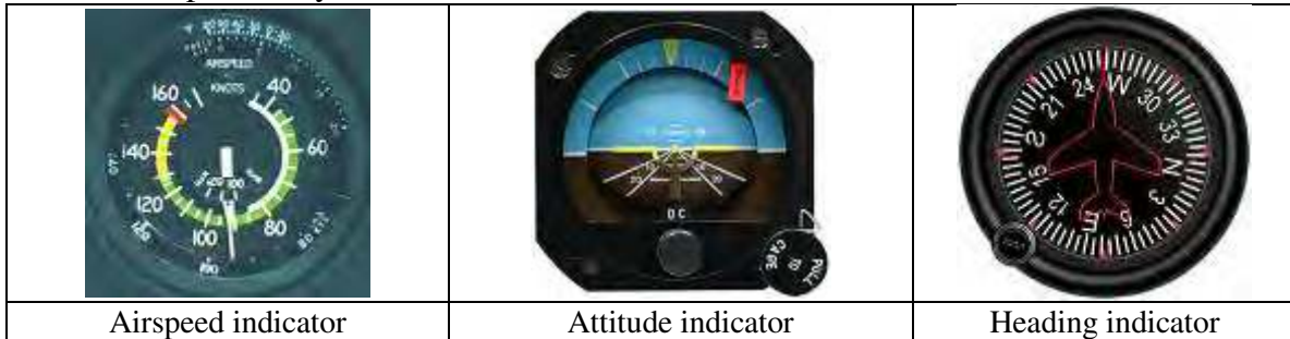
Figure 110. Examples of color in fixed cockpit instruments.
