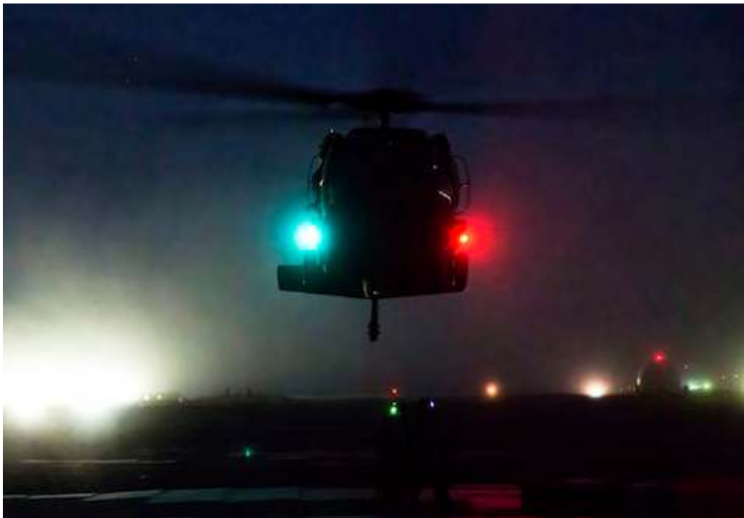
Figure 94. Green and red position lights on UH-60 Blackhawk.
