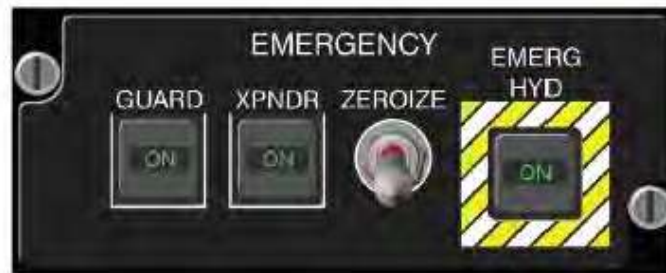
Figure 186. Yellow-white banding around EMERG HYD button on the Emergency Panel in AH-64D that provides hydraulic power.
