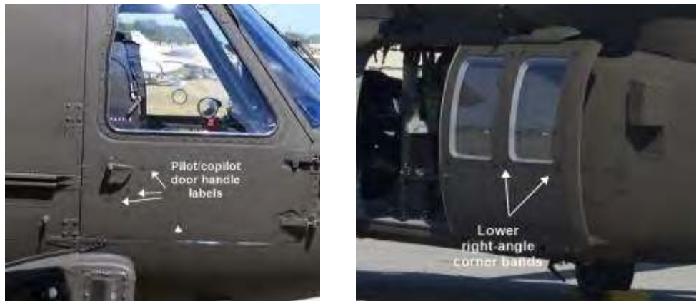
Figure 89. Pilot/copilot door handle exterior labels (left) and rescue panel corner markings (right) on the UH-60M Blackhawk.
