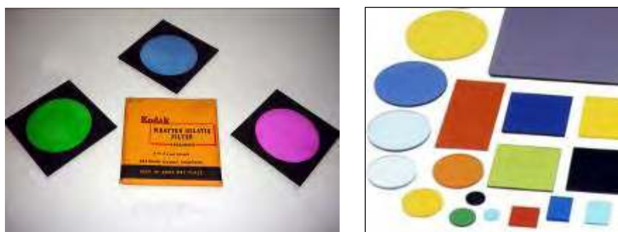
Figure 62. Examples of Kodak Wratten photographic (left) and generic absorptive color (right) filters.
