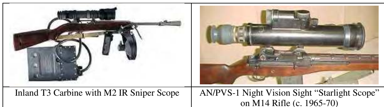
Figure 162. Night fighting weapons: Inland T3 Carbine with M2 IR Sniper Scope (left) and AN/PVS-1 Night Vision Sight "Starlight Scope" on M14 Rifle (right).
