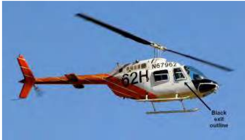
Figure 87. Black emergency egress markings on the U.S. Army TH-67 Creek training helicopter.
