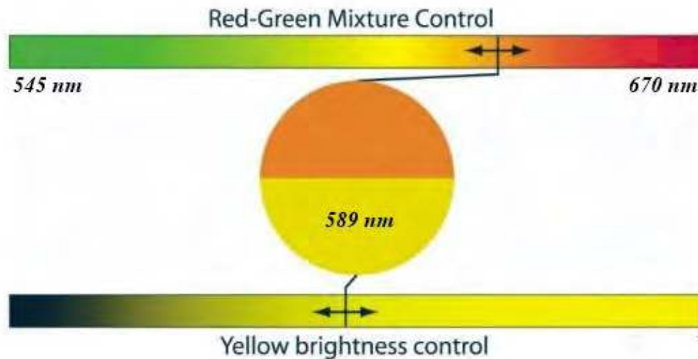
Figure 154. View through the eyepiece of an anomaloscope.
