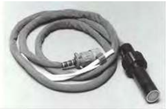
Miniature P-43 based CRT used in IHADSS
