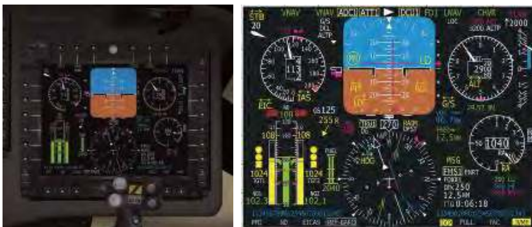
Figure 111. Primary Flight Display (PFD) in U.S. Army's UH-60M Blackhawk, configured for critical flight information.
