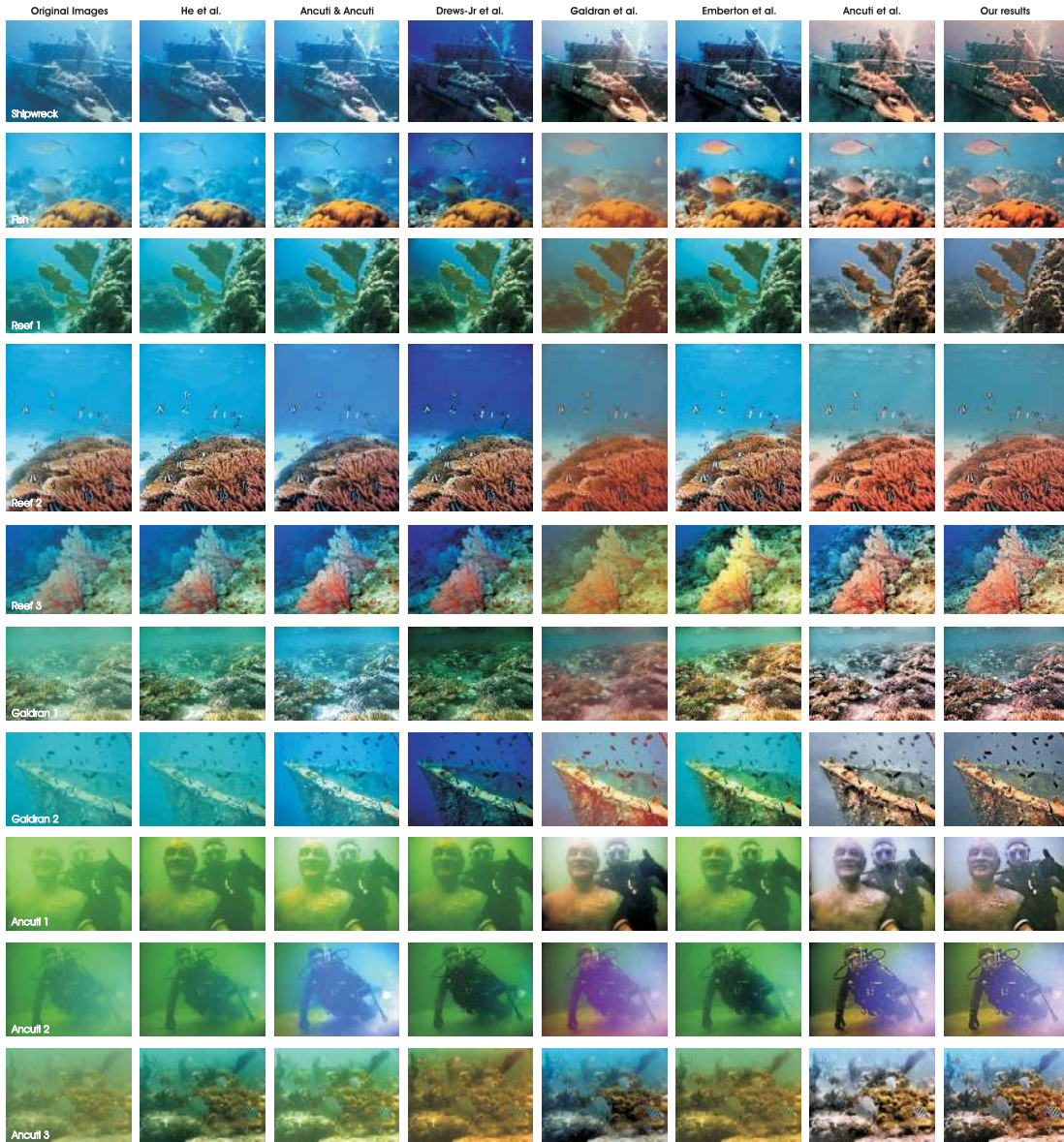
Fig. 10. Comparison to different outdoor (He et al. [19] and Ancuti and Ancuti [23]) and underwater dehazing approaches (Drews, Jr., et al. [28], Galdran et al. [29], Emberton et al. [30] and our initial underwater approach [35]). The quantitative evaluation associated to these images is provided in Table II.
