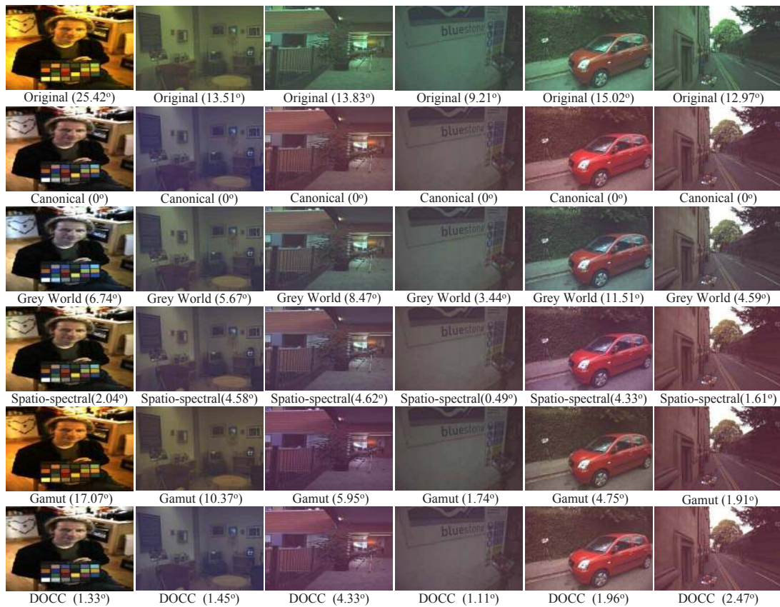
Fig. 9: Some examples of indoor and outdoor images from Gehler-Shi dataset corrected with multiple methods.
