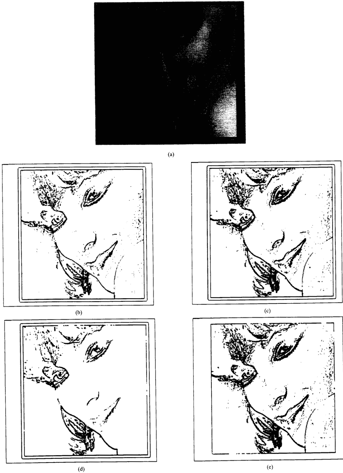
Fig. 5. Edge detection results. (a) Original image, (b) MVD, (c) vector gradient, (d) entropy, (e) vector sum of gradients.
