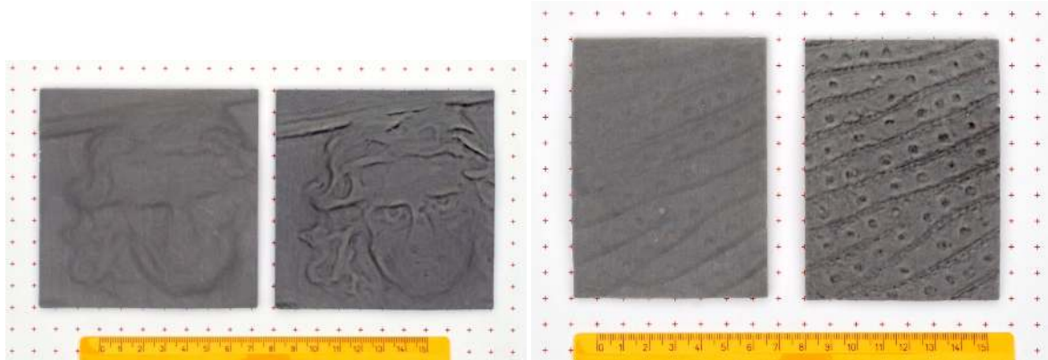
Figure 7: The color-enhancing technique applied to two models that were reconstructed from SEM data. In this case a directionally biased ambient occlusion term allows to start from a lighting that was similar to the standard 'grazing light' approach that is used to better see tiny details raising from a surface.
