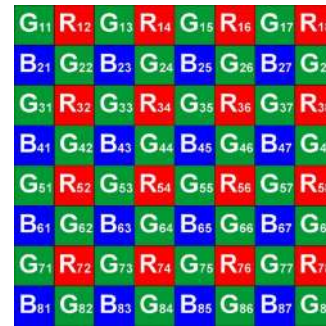
Fig. 1. An 8 \times 8 window of the Bayer pattern.
