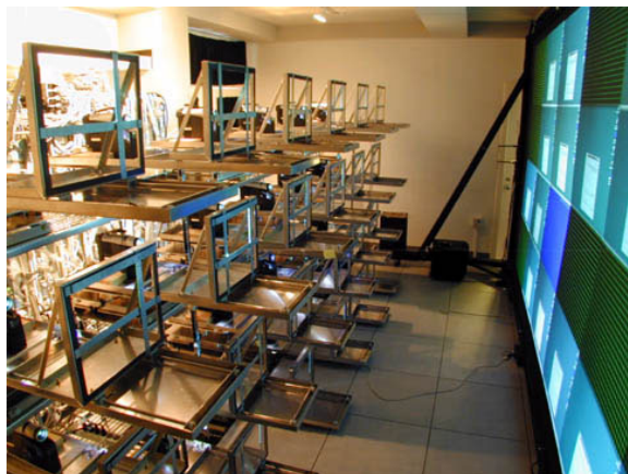
Figure 1: Princeton Scalable Display Wall. There are 24 DLP projectors giving an overall resolution of 6000×3000.
