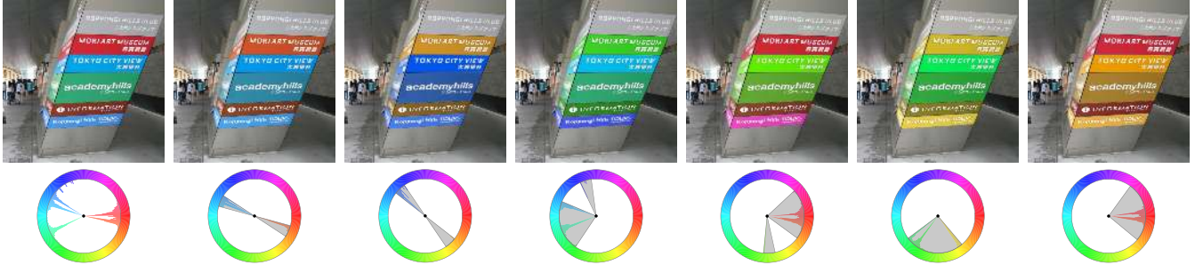
Figure 4: Manual choice of harmonic schemes. The original image and its hue histogram are displayed in the left column. Harmonic templates with various orientations result in different palettes.
