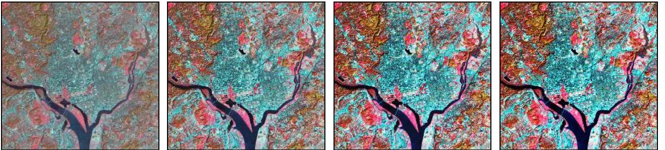
Figure 2. Color histogram equalization (from left to right): the original image, our median equalization ( K=2 ), our quartile equalization ( K=4 ), and exact histogram equalization. This example uses the standard RGB color space. In remote sensing applications, colors are often artificially exaggerated to improve the contrast between image features.
