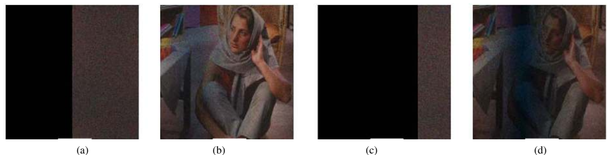
Figure 4. Test of occlusion attack: (a) encoded image with 50% occlusion; (b) corresponding reconstructed image with all accurate keys; (c) encoded image with 75% occlusion; (d) corresponding reconstructed image with all exact keys.
