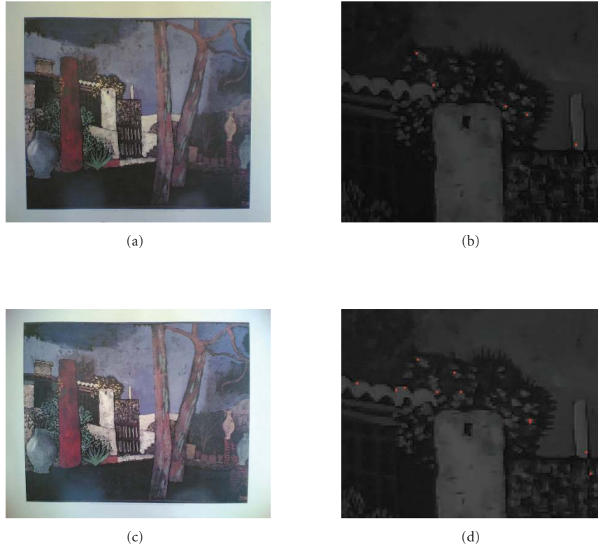
FIGURE 6: Left, sample scene photographed by different cameras (7610 on top, 6681 on bottom). Right, false positives of zoomed-in region of image shown in red. This example illustrates the similarity of the pattern of false positives between cameras.
